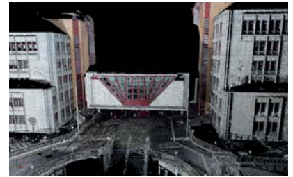
automatically cleaned-up point cloud
