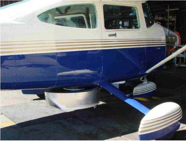
Installation of the fairing in a Cessna 182 Nov 2006
