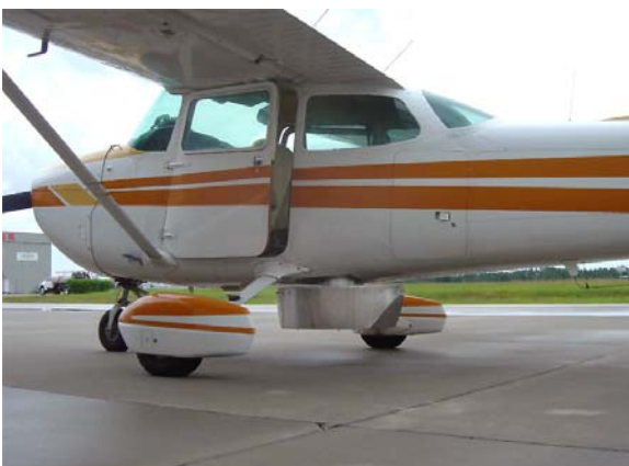
The MIDAS camera pod under a Cessna 172
