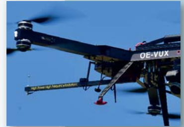
RICOPTER-M equipped with ADS-B/Mode-S transponder
