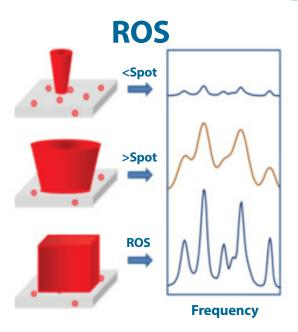
A tightly focused beam may give noisy signals or miss the Raman active target completely. This leads to false negatives from unidentified samples.
