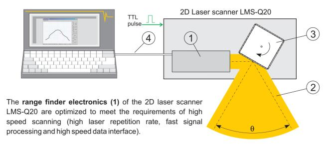
The angular deflection of the **laser beam (2)** is realized by a **rotating polygon (3)** with a number of reflective surfaces. It continuously rotates at an adjustable speed to provide unidirectional scans within an angular range of  $\theta = 90^{\circ}$ .
