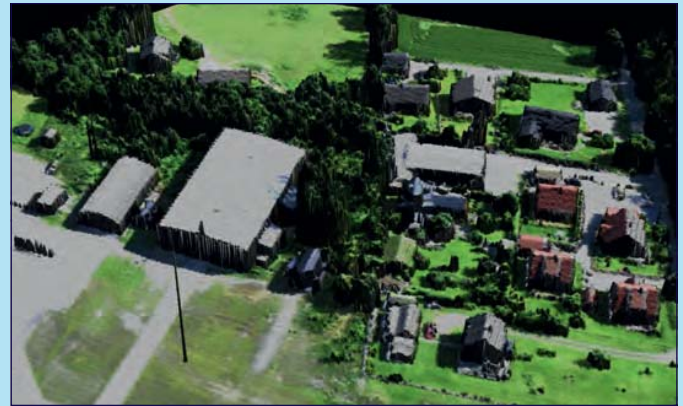
Figure 7. 3D image generated by the combination of a HySpex image and LIDAR data from the same scene.
