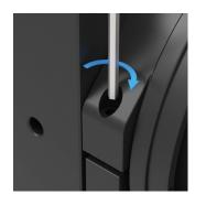
**NB:** Do not overtighten as damage to the lens mount may occur
