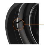
Before mounting a lens ensure the plastic collar is in position and the joint is aligned with the location lug.
