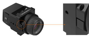
Insert the supplied 2.5mm Allen key into the bolt and rotate clockwise half a turn to engage the lens mount lock.
