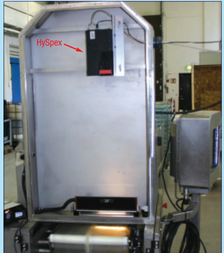
Figure 13. A HySpex camera mounted above a conveyer belt in an industrial application.
