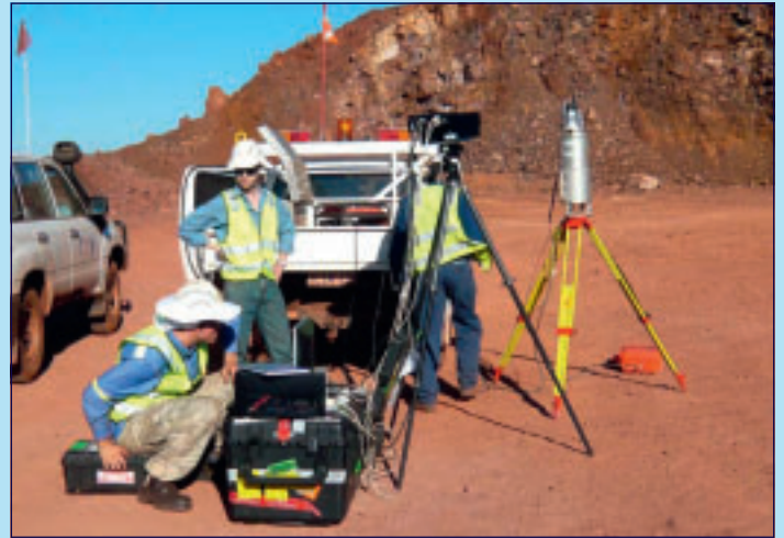
Figure 10. HySpex camera and LIDAR set up for mine face scanning.
