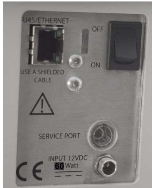
Figure 2-6 AgriSpec spectrometer back panel showing Ethernet connection, power switch, and power input jack.
