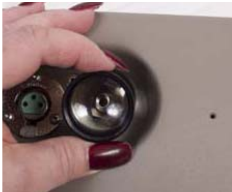
Figure 4-9 Internal spectrometer LED shining to test internal fiber optic cable.
