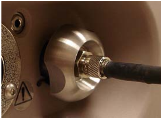
Figure 4-3 View of the fiberoptic cable, fiber bundle matcher, and fiber connection. Screw the fiber bundle matcher into the fiber connection as far as possible.
