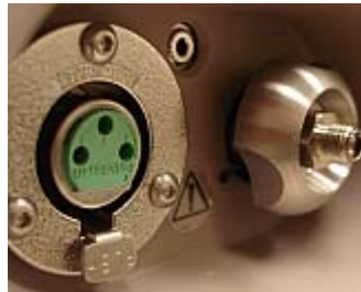
Figure 4-2 View of the fiber optic bundle matcher and the fiber optic port.
