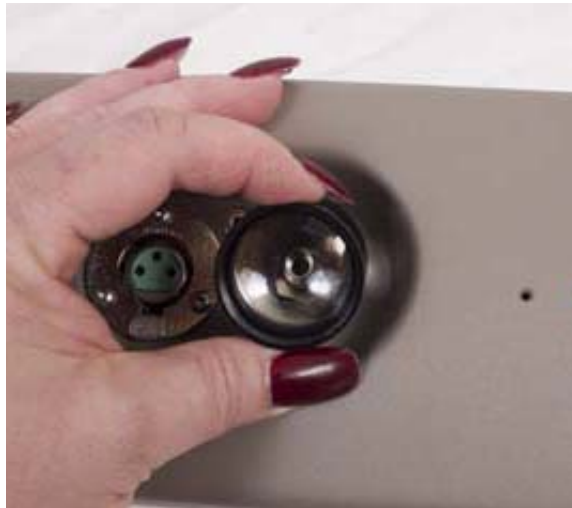
Figure 4-10 Internal spectrometer LED shining to test internal fiber optic cable.
