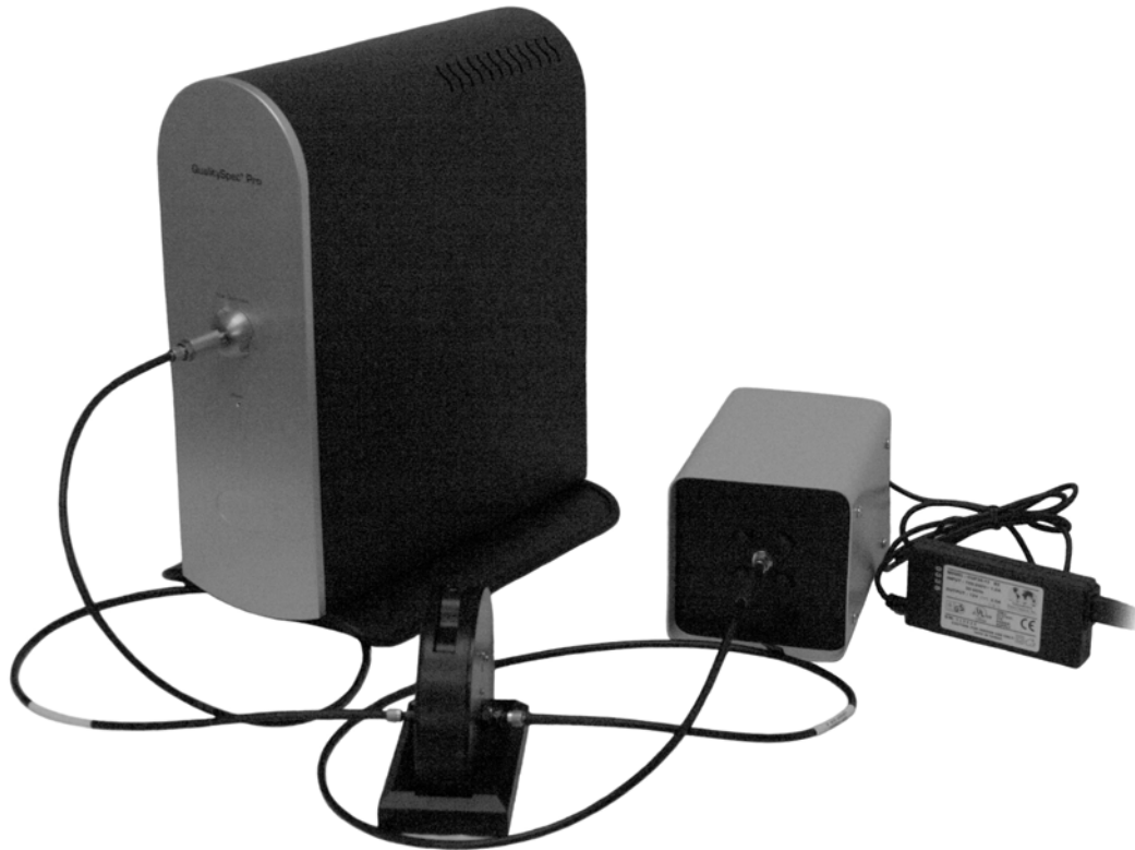
Figure 4-4 QualitySpec spectrometer front-view showing fiber connection to USP filter wheel and light box.
