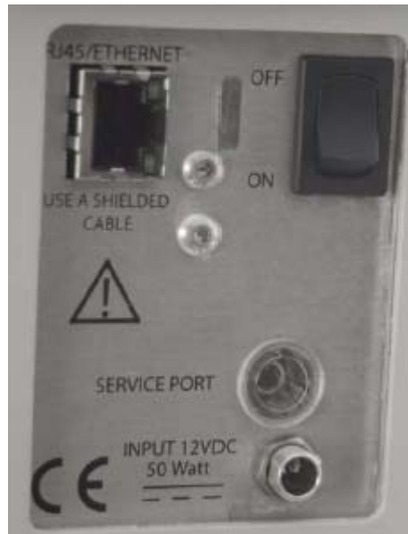
Figure 2-5 QualitySpec spectrometer back panel showing Ethernet connection, power switch, and power input jack.
