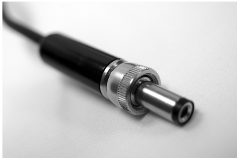
Figure 2-4 QualitySpec spectrometer power connector which plugs into the instrument.
