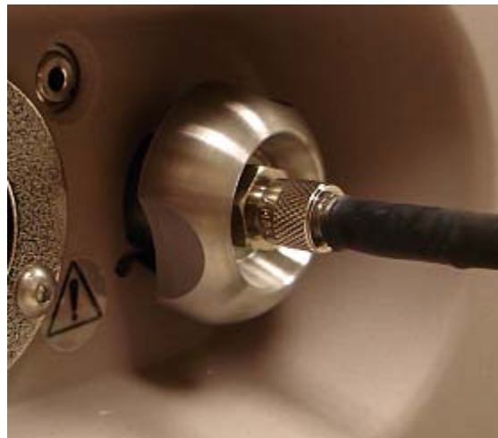
Figure 4-3 View of the fiber optic cable, fiber bundle matcher, and fiber connection. The fiber bundle matcher should be screwed into the fiber connection as far as possible.
