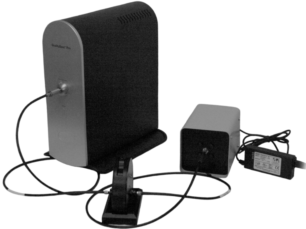
Figure 2-2 QualitySpec spectrometer front-view showing fiber connection to USP filter wheel and light box.
