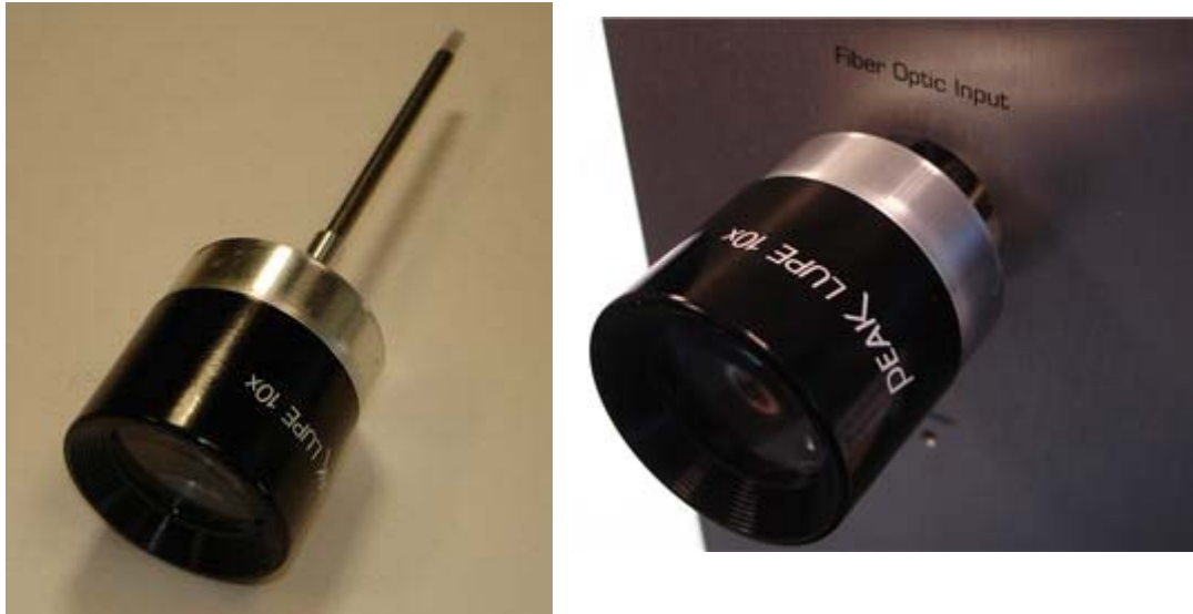
Figure 4-8 Magnifier for testing the internal fiber optic cable.
