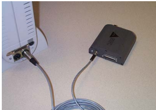
Figure 6-3 ASD Smart Ethernet Adapter showing the power cable connected to the instrument.
