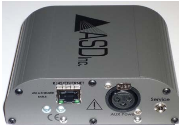
Figure 6-13 Enhanced view of the accessory power jack for probe.
