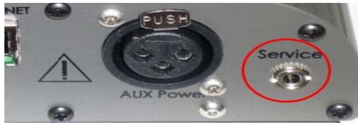
Figure 6-14 Enhanced view of the serial port.
