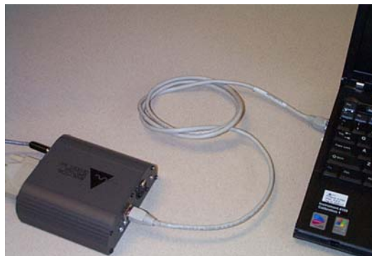
Figure 6-2 ASD Smart Ethernet Adapter showing the cross over Ethernet cable connected to the instrument controller.
